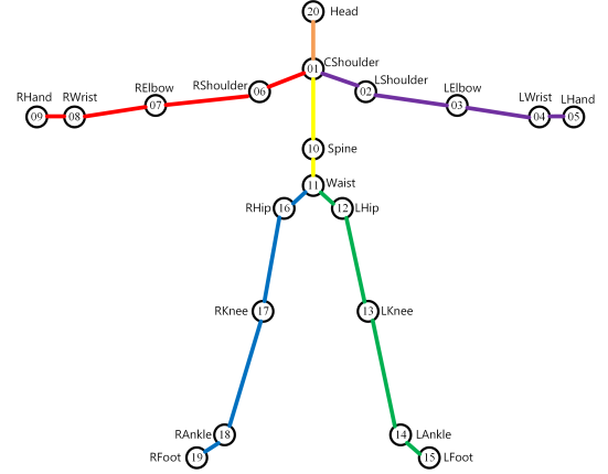
Figure 4: Standard human model of 20 body skeletons marked by black spheres and 6 body components marked by colored line segments: Torso, Head, LArm, RArm, LLeg, RLeg. The parent relationship of all nodes of the tree is given by (1).
