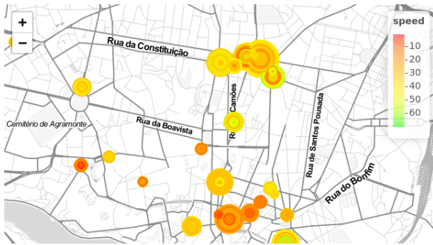
Figure 3: Global Visual Exploration View: traffic speed and volume represented by circle color and radius, respectively.
