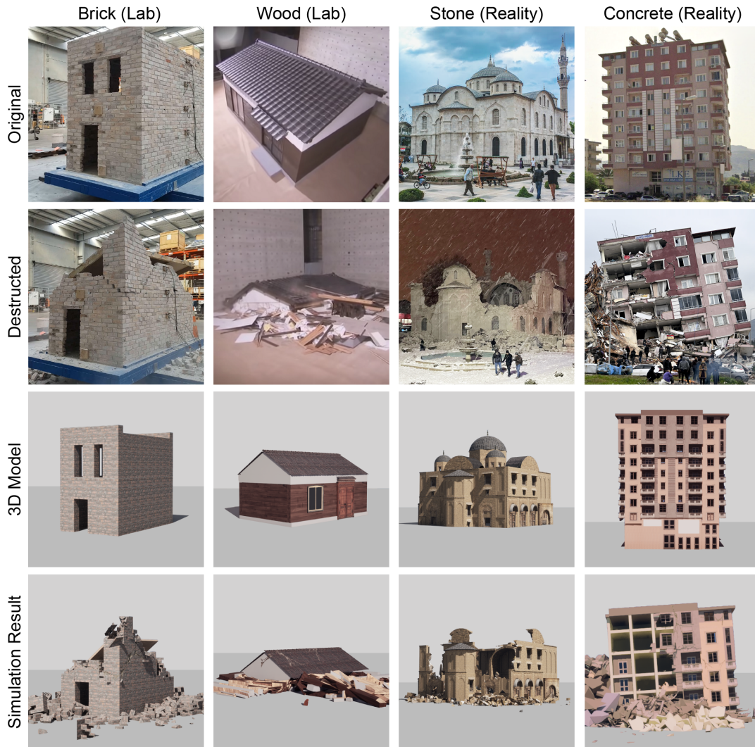
Figure 6: Earthquake simulation using RESEnv for four actual scenarios. Two laboratory experiments (columns 1-2) and two actual buildings (columns 3-4) were chosen. Row 1: The original forms of four buildings before the earthquake events. Row 2: Destruction of buildings following the earthquake events. Row 3: The 3D models are recreated based on the actual buildings and are given textures and pre-fracture settings in RESEnv. Row 4: Destruction results of four buildings after RESEnv earthquake simulation.
