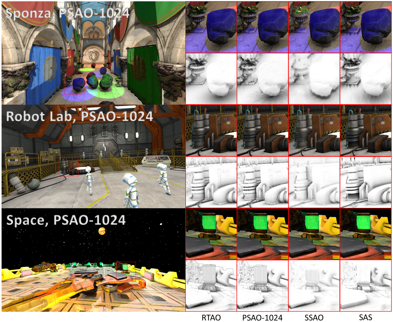
Figure 4: Qualitative comparison of rendered frames between PSAO using 1024 points per unit area, ray-traced per-pixel ambient occlusion (RTAO), SSAO and SAS.
