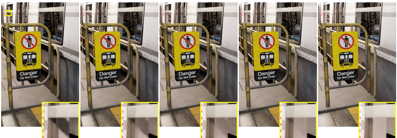
Figure 16: Denoised results in the Subway scene, changing the per-pixel rays counts by reusing visibility for nearby neighbors. The intuition: when reusing lights from distant pixels, visibility is more likely to change. Left-to-right: 2 rays per pixel (no reuse), 1.75 rays per pixel (reuse within 15-pixel radius), 1.5 rays per pixel (20-pixel radius), 1.25 rays per pixel (25-pixel radius), and 1 ray per pixel (always reuse).
