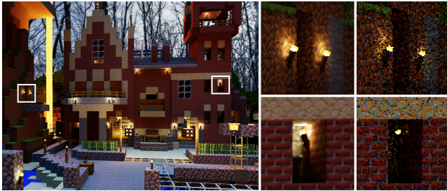
Figure 20: Resampling can undersample very complex lighting. A reference with insets, (left) reference and (right) ReSTIR, of the extensive “Vokselia” Minecraft world with 200,000 emissives, mostly torches with limited range. Torch lighting flickers temporally, as pixels rarely find a relevant light; when a torch is proposed as a candidate, it is rarely at a pixel within range of the torchlight.
