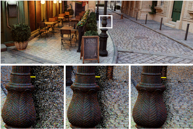
Figure 11: The Amazon Bistro (top) with insets showing temporal disocclusions under horizontal motion, using three settings. (Left) Temporal reuse only, (center) temporal reuse plus one spatial sample, and (right) temporal reuse plus five spatial samples. The yellow lines show the width of the disocclusion in one frame.
