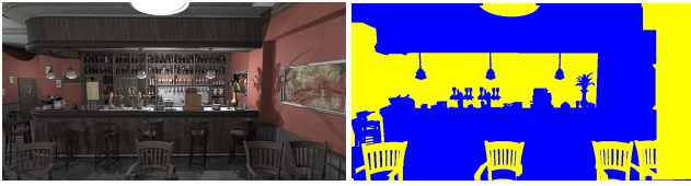
Figure 9: An example of the scene segmentation during strictly horizontal motion, where a yellow pixel indicates that its tile is rendered with the hourglass pattern, while a blue pixel indicates that its tile is rendered with the bowtie pattern.
