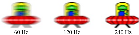
Figure 2: Motion blur reduction with 240 Hz, at 960 pixel per second motion. Images courtesy of Blur Busters [Rej13].
