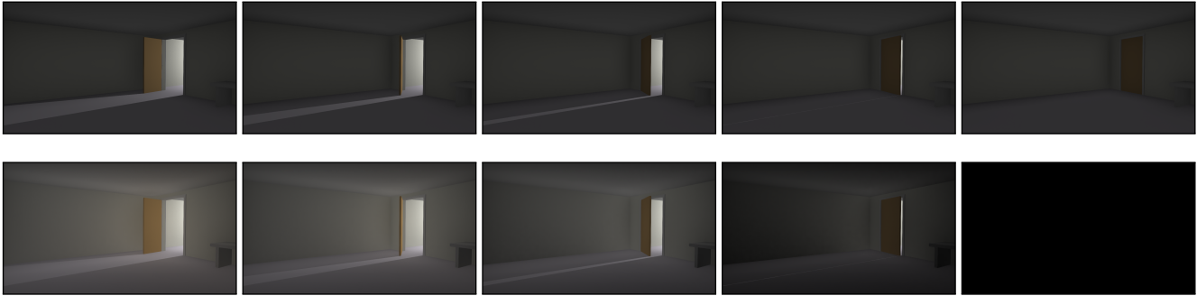
Figure 1: Screen-space radiosity (bottom) can capture simple dynamic illumination phenomena well compared to a static environment map probe (top). We show a completely unlit room with a door to a very bright adjacent door as the door closes through multiple frames of animation.
