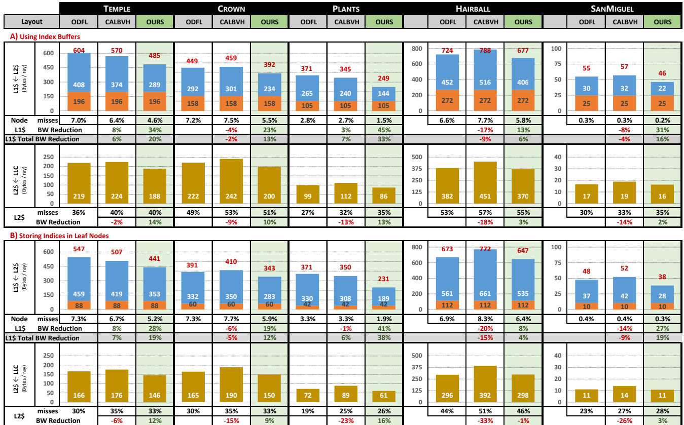
Figure 8: General bandwidth measurements on all test scenes. The cache sizes were: Node L1 40 KB, L2 256 KB, Triangle L1 32 KB. On the L1 bus we color-coded the triangle-bandwidth in orange and the node-bandwidth in blue. We can observe a major improvement in bandwidth when the indices are stored in leaf nodes.
