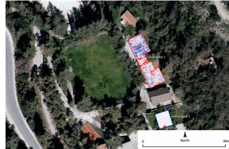
Figure 2: Ground Penetrating Radar Survey, Time-Slice, Agios Nikolaos tis Tegis, Kakopetria, Cyprus.
