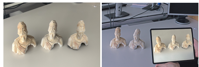
Figure 7: Left image (from left to right): Original object, 3D printed replica, and 3D rendered virtual model. Right image: Photo of real scene and AR view on iPad.
