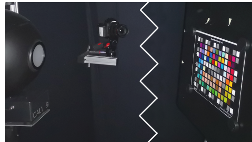
Figure 4: Setup used for capturing color data: Color checker with known spectral data is captured to estimate the transform matrix.
