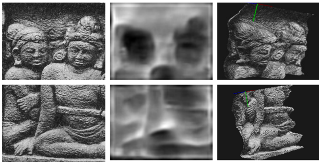
Figure 3: Details of the 3D reconstruction results (from left to right): monocular photo patch, depth prediction map, and the reconstructed result.
