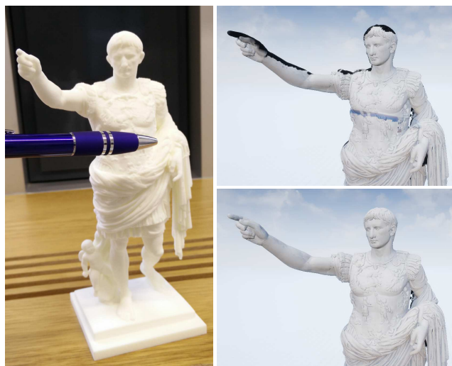
Figure 9: Due to depth-tracking-based imprecision, depth-based culling misses parts of the occluding pen and crops the model’s silhouette (top right). These artifacts are removed when dilating the depth image from the depth camera (bottom right).
