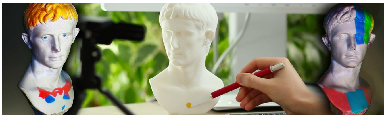
Figure 1: Proxy painting enables artists to paint onto a proxy object (center) in a permanent (real paint) or nonpermanent (digital paint) way. The painting is projected onto the original unmodified target object using projection mapping (left, right).
