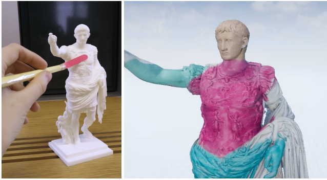
Figure 5: A pointing device with a colorful tip is held close to the proxy object. The color is recorded and applied to the model.
