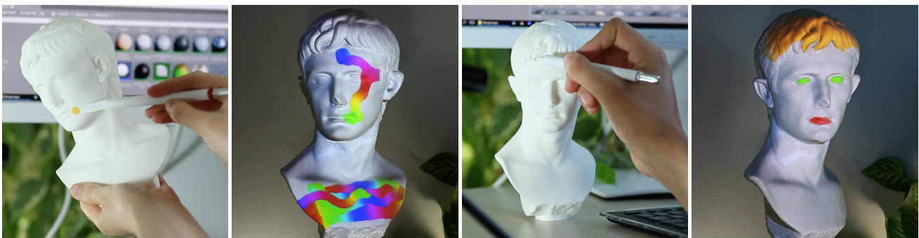
Figure 13: In the 3D Graphics Tablet mode, the user touches the proxy with a registered yellow dummy brush (different tip sizes). The actual painting color is set digitally (e.g. multicolored in the left example). No artifacts are caused by the artist's fingers or the dummy brush.
