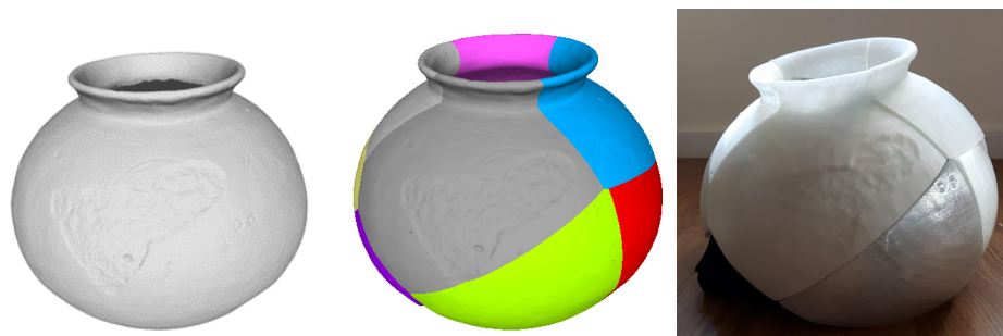
Figure 1: a) 3D scanned model of pottery urn artefact; b) 3D model of puzzle pieces of reconstructed urn; c) printed parts of the puzzle
