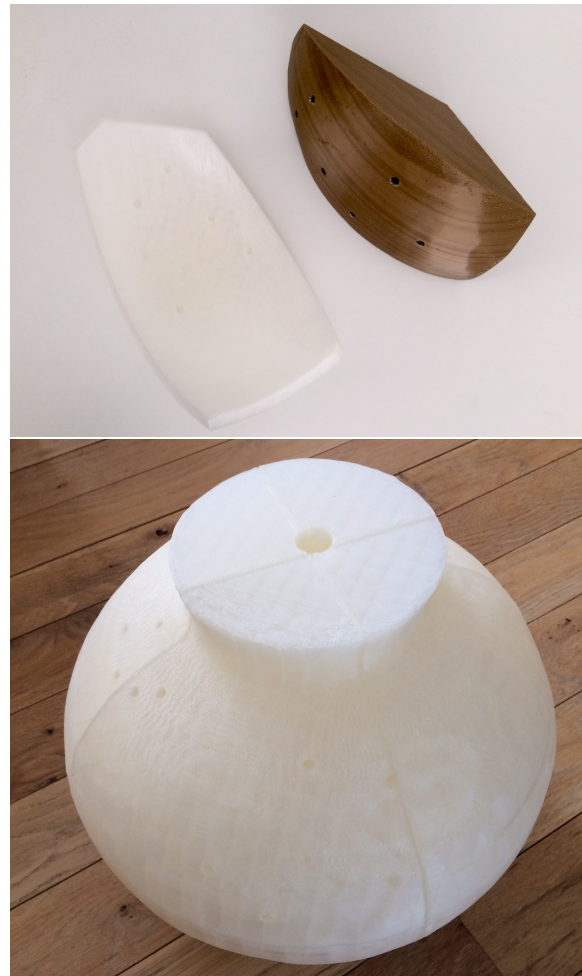
Figure 12: a) 3D printed set of samples with cylinders generated using as input a set of points in 3D space; and b) printed core piece
