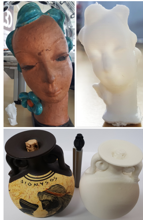
Figure 6: Comparison of original objects with their 3D printed replica. Top: 'Bust' printed at scale 12% on Dremel 3D40 (enlarged view). Bottom: 'Greek Vase' printed at scales 18% (black) and 95% (white) on Ultimaker 2+.
