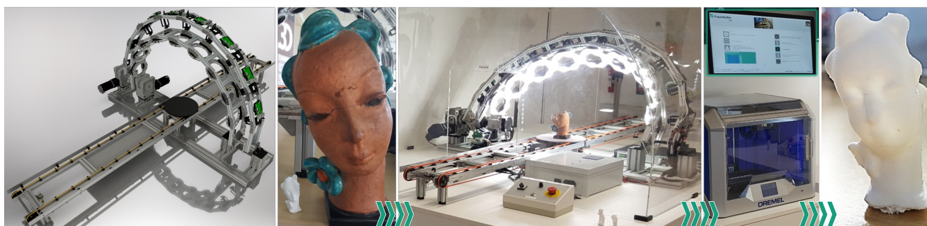
Figure 1: CultArc3D_mini CAD design and automatic process flow from artifact over 3D scan and 3D reconstruction to 3D print of replica.
