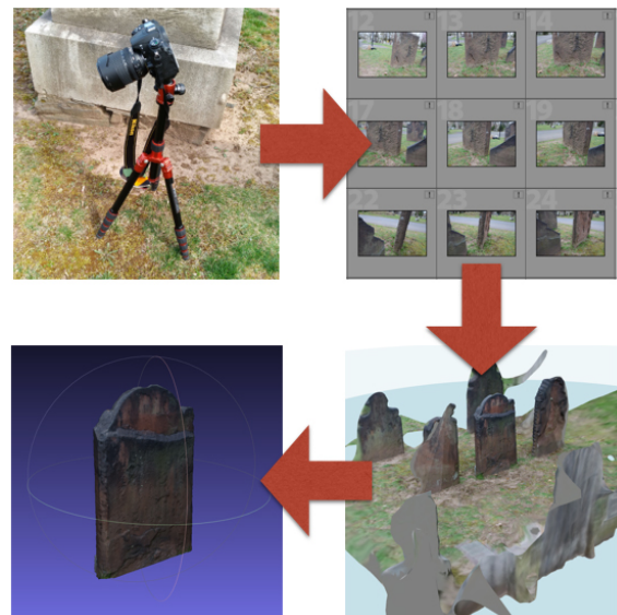
Figure 2: Our method requires an isolated 3D manifold model to work properly. Generating it consists on taking the pictures, loading them to Autodesk ReMake, which generates a 3D reconstructed scene and, then, separating the target model and filling its holes.
