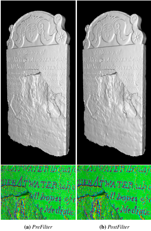
Figure 3: We perform a smoothing filter to reduce the acquisition noise of the reconstructed model. Here it is shown a comparison before and after applying the filter (top) and zoom-in's showing the obtained color-coded curvature in each case (bottom).
