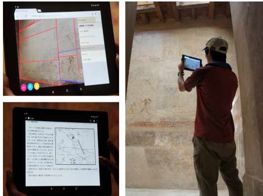
Figure 7: AR use on a mobile tablet; photo shooting situation (right), AR representation onto a live photo (top left) and retrieved information (bottom left)
