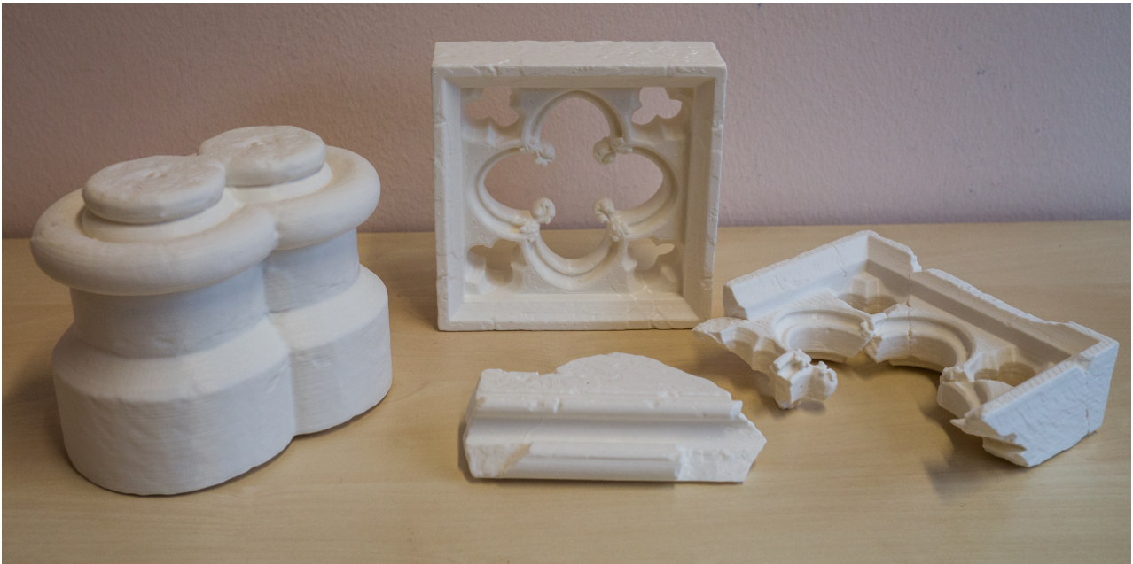
Figure 9: A collection of 3D printed results produced by our method from left to right: reassembled column based with restored fracture lines, reassembled and completed embrasure fragments with restored fracture lines (top), reassembled arch with restored fracture lines (bottom), and reassembled and merged embrasure fragments with unconcealed fracture lines.
