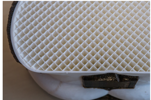
Figure 7: Thin grid supporting the inside of a partially printed column base object. On the outside, part of the external support structure is also visible.
