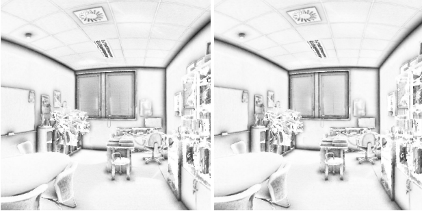
Figure 4: Multi View Ambient Occlusion with different maximum depth threshold d_{max} in Equation 10: (Left) d_{max} = 2m ; (Right) d_{max} = 6m .
