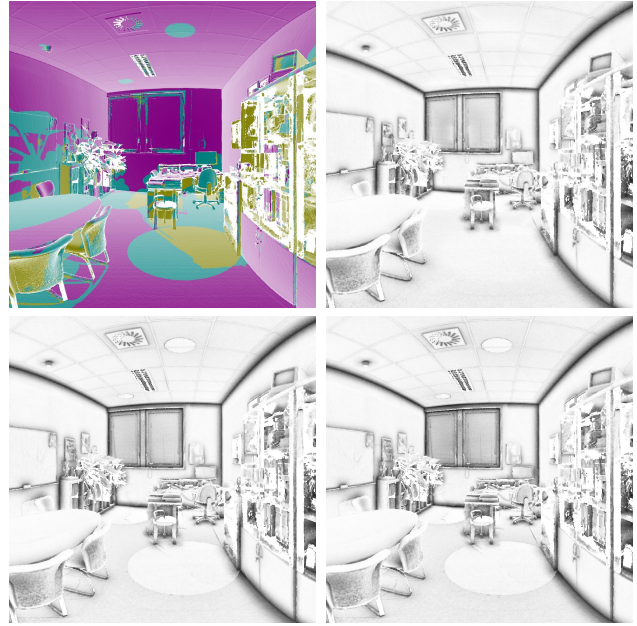
Figure 5: Effect of the border weight w_b on the computation of the MVAO: (Top-left) image with the color encoding of the scan coverage for each point (yellow = one scan, light blue = two scans, pink = three scans); (Top-right) MVAO using our weighting function in Equation 9; (Bottom-left) MVAO using the weighting function proposed in [VPG13]; (Bottom-right) MVAO using our weighting function without the border weight w_b .
