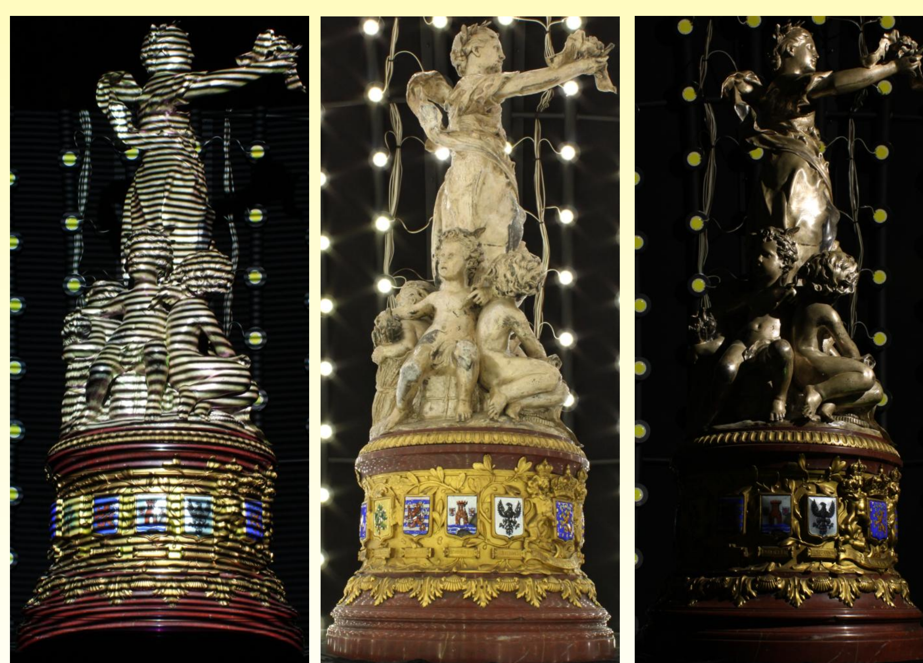
Figure 3: Exemplary raw data (left to right): Fringe image, shadow-free image, reflectance image
