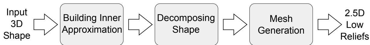
Figure 1: Overview of the pipeline stages to convert a 3D model into a set of interlocking pieces.
