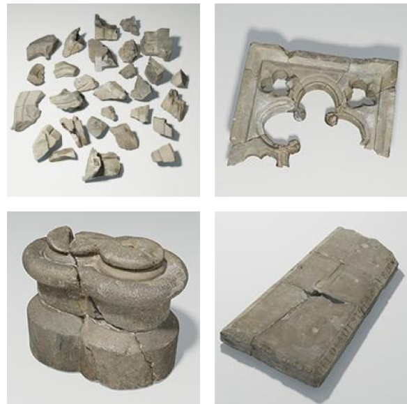
Figure 1: Defective objects from Nidaros Cathedral, Trondheim, Norway: Fragments of a doorway arch (top left), reassembled embrasure with missing parts and cracks (top right), reassembled column base with large cracks (bottom left), reassembled tombstone with hole and cracks (bottom right).
