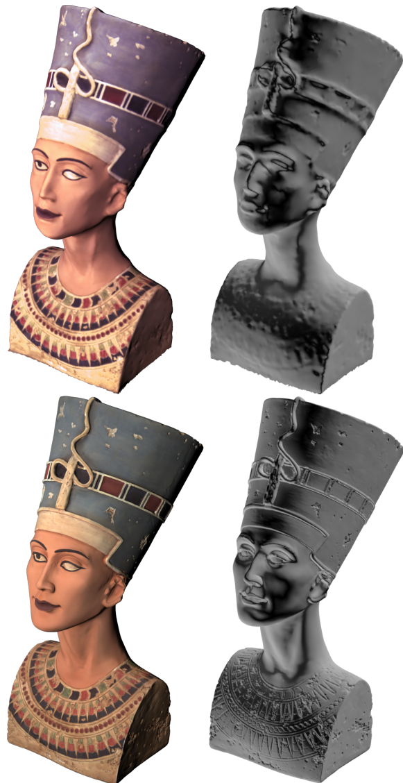
Figure 7: Comparison of the resulting 3D models from scanning a reproduction of a Nefertiti bust with the CultArc3D system (top row) and with a structured-light scanner (bottom row), textured (left) and gray shaded (right).
