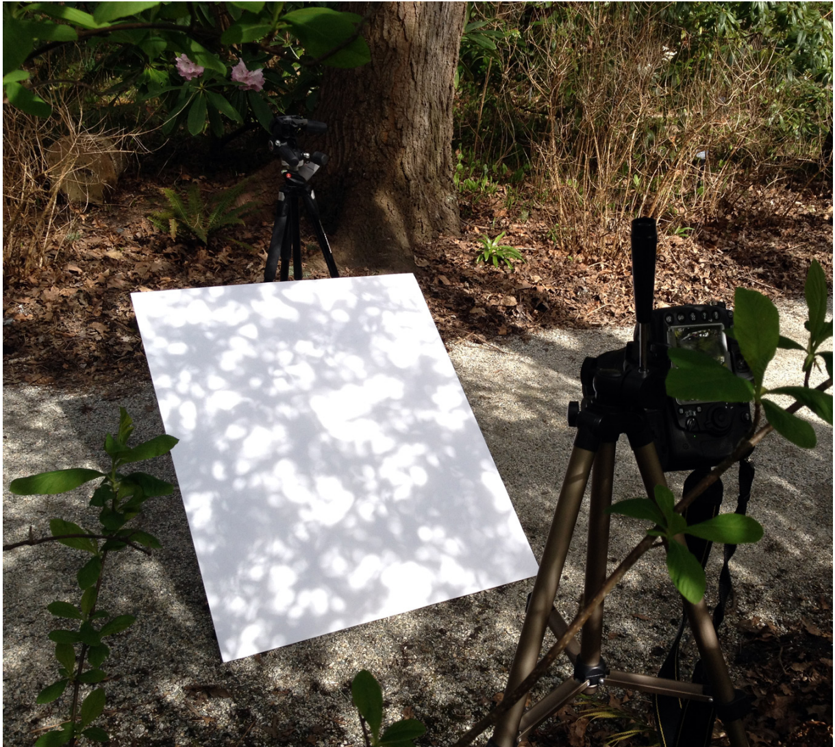
Figure 5: Field study setup of the foliage shadows in real life. Circular light spots appear on the white foam core board at a proper distance. We aligned the foam core board to be orthogonal to the direction of the sun shine. If the shadow receiving plane is not orthogonal to the direction of light (such as the ground), the light spots will be elliptical.
