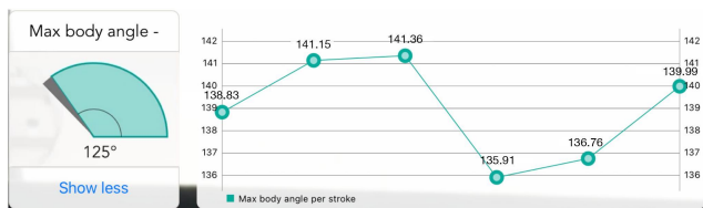
Figure 2: Finish body angle. Left: The arc diagram shows the current finish angle, highlighting the difference to the previous stroke's finish angle (grey area). Right: Finish body angle over time.
