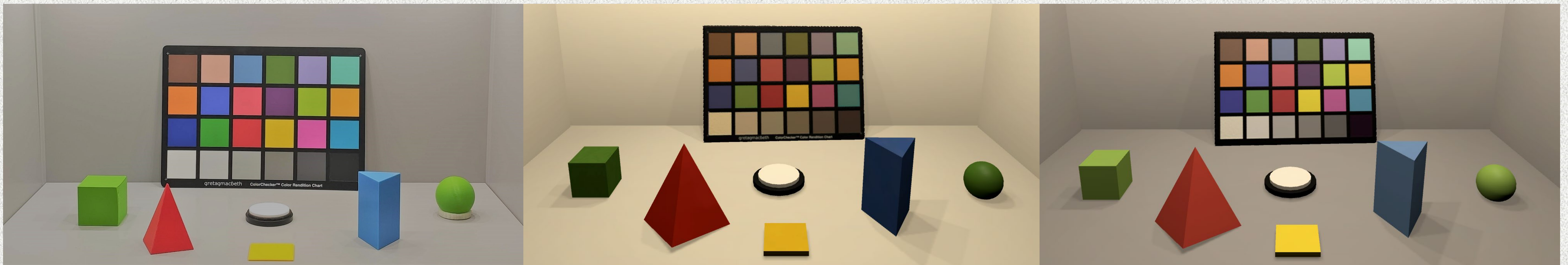
Figure 1: The quantitative experimental environment. Left: Scenario on a real light booth and real several objects created with a 3D printer; Center: Virtual environment with 3D scanned objects and RGB textures under D50 illuminant; Right: Virtual environment with 3D scanned objects and hyperspectral textures under D50 illuminant.
