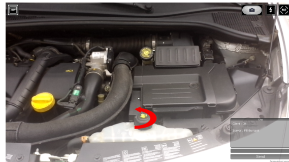
Figure 7: The unskilled operator receives via chat the instruction to add water in the tank.
