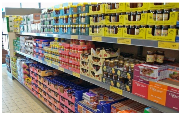
Figure 2: Example of shelf-ready packaging: Corrugated cardboard boxes containing the products-to-sell are placed on the shelf without unpacking.
