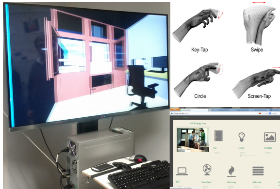
Figure 4: The 3D TV (left), implemented gestures (top right) and the web interface (bottom right).
