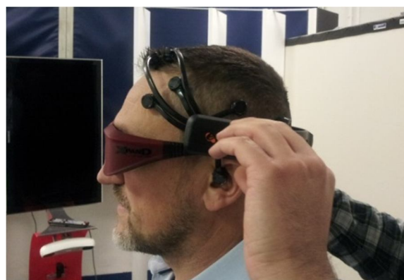
Figure 3: The headset is fitted on the head of the participant for recording the brain waves during the test.
