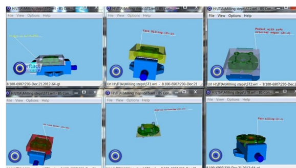
Figure 9: The instructions show first milling operation that should be performed (face milling). These instructions will guide the user through all necessary machining operations until the rough stock becomes the finished part.
