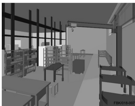
Figure 7: Analysis of the area covered by a virtual crane within a factory layout
