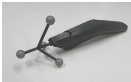
Figure 8: Stylus tool for immersive sketching.
