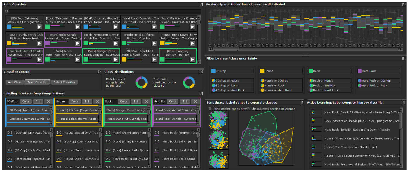
Figure 1: Overview of our system for the personalized visual classification of music collections. Upper left: querying and browsing interface for all songs. Lower left: class creation, labeling, and class prediction interface. Upper right: analysis of features and class distributions. Center right: filtering interface for classes and class collisions. Lower right: two interfaces for the meaningful selection of labeling candidates (based on dimensionality reduction and active learning). Throughout this work, we apply a test dataset for genre classification. Note in our examples, we give the true class label in [brackets] in the song names for verification.
