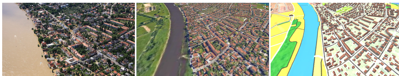
Figure 1: Left: Aerial view of the Laubegast, a district of Dresden, Germany, during the 2013 flood event [Pet13]. Centre: a model of the same region from a similar viewpoint in our Virtual Geographic Environment using high-resolution aerial imagery as texture. Right: The same model with landuse data texture applied.
