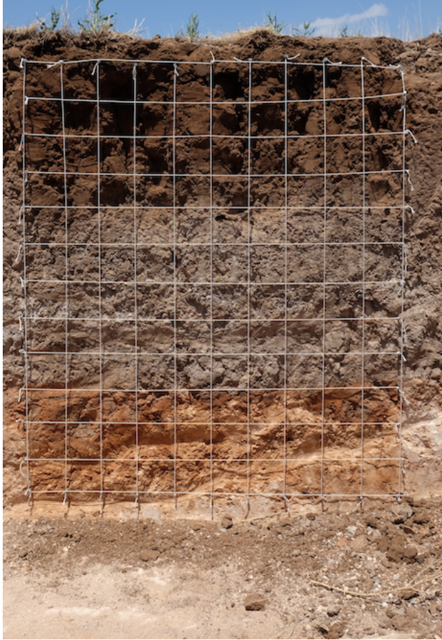
Figure 2: The grid layout of a soil profile: Vertically, there are 13 horizons (named as ‘A’ to ‘M’ from top to bottom correspondingly). Horizontally, there are vertical slices that the soil analysts need to measure (named as ‘1’ to ‘10’ from left to right, respectively). Each grid cell is of size 10 × 10 cm).
