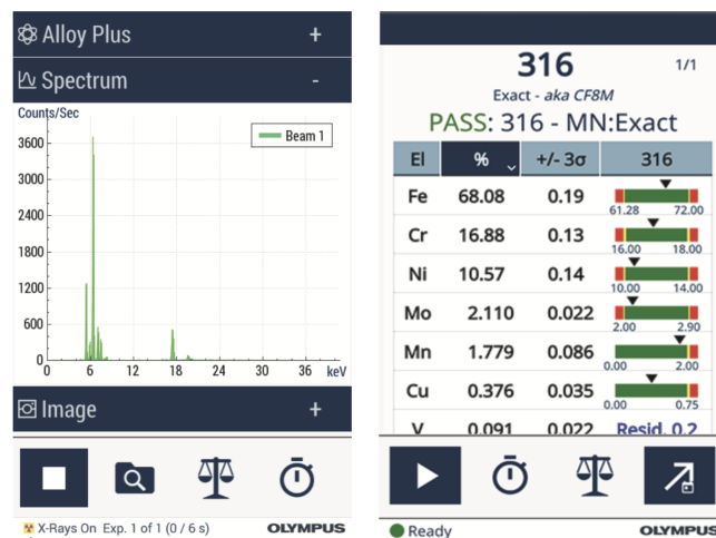
Figure 1: Vanta Handheld XRF series built-in interface. This figure is adapted from Vanta Family X-Ray Fluorescence Analyzer User’s Manual [Ana16].
