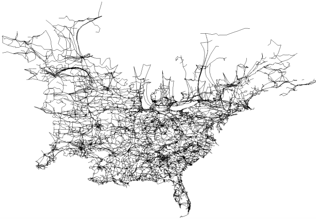
Figure 3: The result of kernel density edge bundling on the Eastern Interconnection [HET12]. Longer transmission lines are moved towards denser parts of the network due to the edge bundling formulation. Since power systems consist of either small lines densely connected together with little overlap, or long lines that, edge bundling techniques are an ill suited visualization technique.
