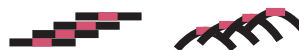
Figure 3: Rendered as disks normal to the viewing direction (downwards), points near each other can form an occluding sequence and appear all black. When rendered as paraboloids (right), like the tapering used in [EBRI09], this is much less likely.
