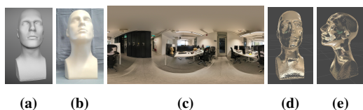
Figure 3: Virtual (a) & real (b) mannequin heads with captured environment map (c) used to generate glass phantom (d), (e)
