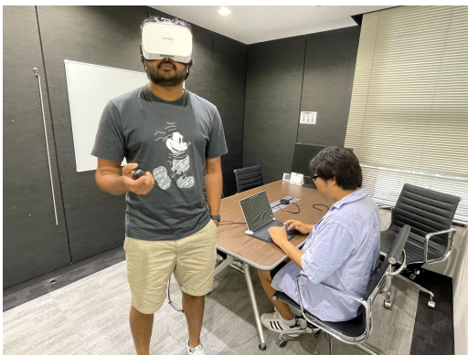
Figure 1: A subject is wearing the HMD in a room. The host PC records his eye-tracking data during the data collection process. He holds a controller with a press-to-teleport button to move in the VR environment.
