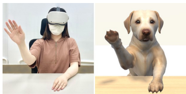
Figure 1: The user wearing an HMD (left) and the dog avatar with movements converted from the user's nonverbal information (right)
