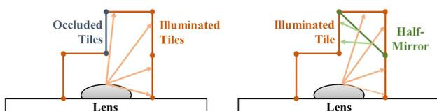
**Figure 15:** An occluded tile (left) can be projected onto by using a half-mirror at the position seen on the right side.
