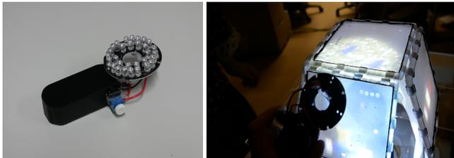
**Figure 7:** The external LED light (left) and an example application where the user can draw textures onto which animals (right).
