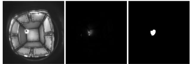
**Figure 8:** The camera input image (left), the background subtraction (center) and the binarized imaged used to detect the light (right).
