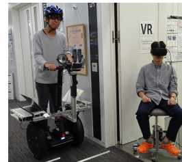
Figure 1: Overview of proposed telepresence system. ( TwinCam Go ) Left: driver on a Segway with TwinCam system, right: viewer on a rotary seat.
