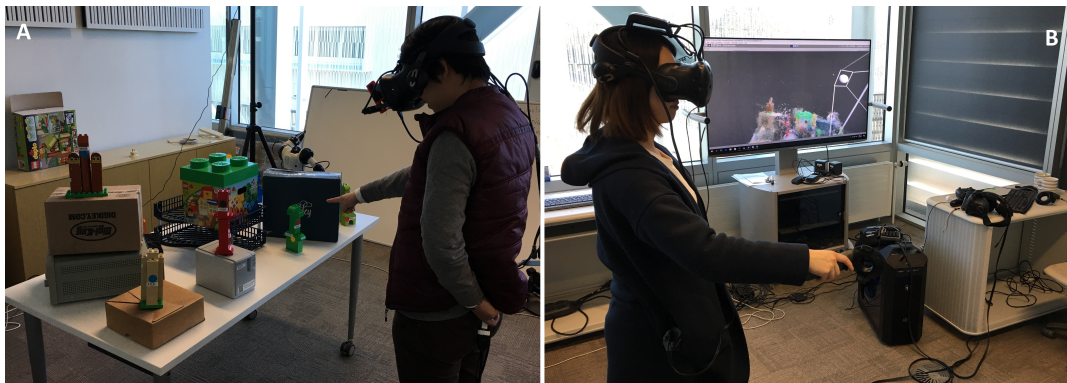
Figure 1: Static local environment capturing with real-time feedback for Mixed Reality remote collaboration. A: the local user stands in front of a workspace, identifying a particular LEGO model which the remote helper has pointed at. B: The remote expert observes the local environment and guides local worker via pointing in the VR world.
