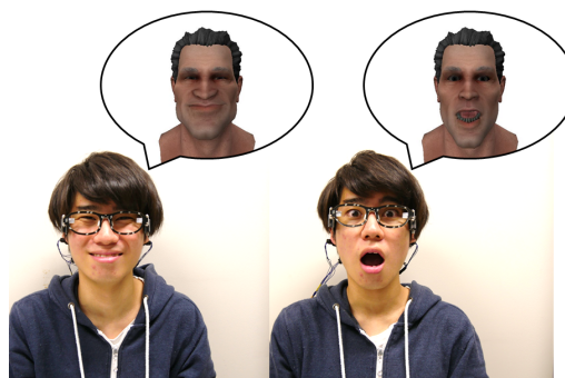
Figure 1: Our system estimates 3D points on the skin surface using smart eyewear. We can retarget the facial expression to the 3D model from the points.
