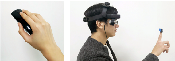
Figure 6: The experimental set up: the air mouse used for Hand-Cursor (left) and the head mounted camera connected to a smart phone for the Blurry Finger / Blurry Finger-Cursor (right).
