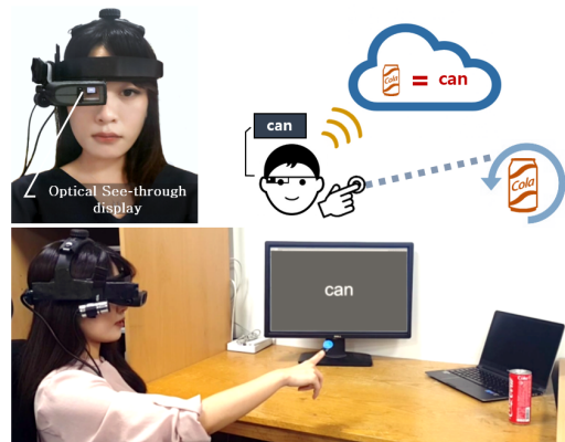
Figure 12: The Blurry Finger based AR based image searching system: (top) system set up with the OST display and (below) a scene from actual usage. The result on the OST display was also shown on the monitor
