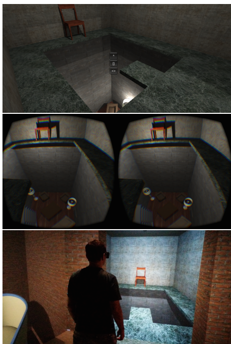
Figure 2: A Virtual Pit loaded on three different Decks. Top: screenshot of desktop client. Middle: screenshot of HMD client. Bottom: view of user inside the CAVE.
