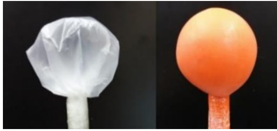
Figure 6: Balloon structure (left: inner bag made of polyethylene, right: rubber balloon used as outer bag)
