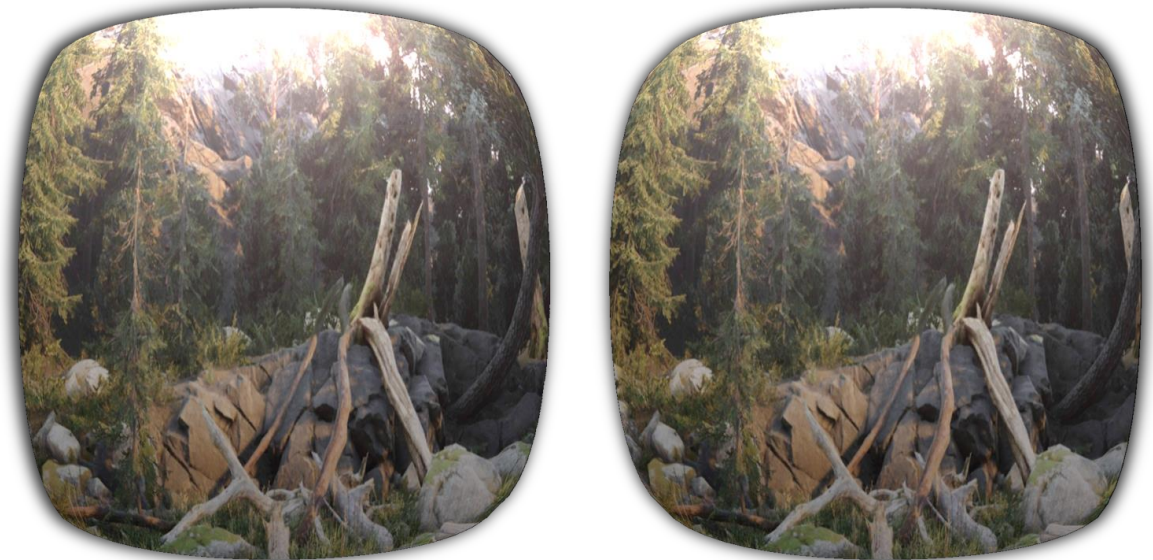
Example of barrel-distorted HMD stereo rendering
