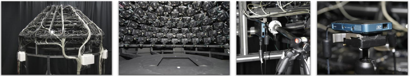
Figure 29: Multiview BTF acquisition device used in [MMS*04, SWRK11]: An array of 151 cameras on the upper hemisphere above the object allows a highly-parallelized acquisition. The camera flashes have been used as light sources so that a dense sampling of 22,801 view-light configurations can be achieved. The use of projectors in the setup as used in [WSRK11, SWRK11] allows a structured light based geometry reconstruction.
