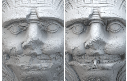
Figure 24: Comparison of different surface reconstruction methods. Left : A global approach by [MKG11]. Right : An approach based on a local implicit function [FG14].
