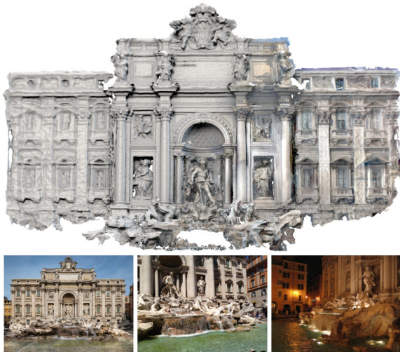
Figure 41: Reconstruction by MVE [FLG14] of an Internet dataset downloaded from Flickr. The bottom row shows 3 images of a total of 871 input images. The top row shows the reconstruction rendered with shading (left) and with texture (right). Photo credits: Flickr users Vince O'Sullivan , Andy Hay , Ecyrd , Creative Commons License
