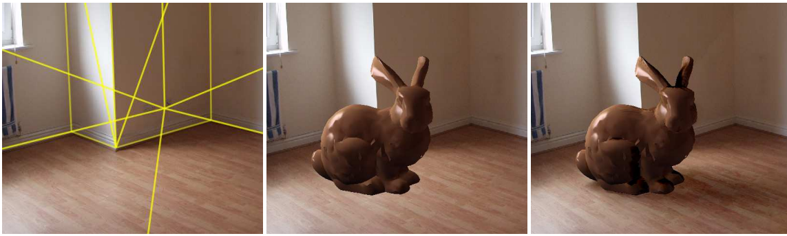
Figure 2: Overview of the rendering process. From the calibrated camera position corresponding to the background image (top), the reconstructed scene geometry is drawn into the depth buffer and synthetic objects are rendered into the color and depth buffers to resolve occlusions (middle). Finally, multiple shadow passes are performed, blending shadows into the composited image (bottom). For this example, the image on the right was generated at over 9 frames per second.
