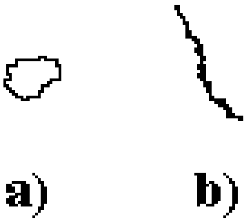
Figure 6: Two kinds of degradation belonging to the class of lack of material: a cavity (left) and a fissure (right).
